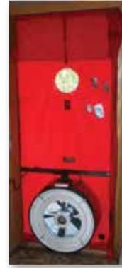
A blower door test uses a fan to pressurize and depressurize your house to detect leaks. Common areas for leaks are around window and door frames, recessed ceiling lights, electrical outlets, and plumbing underneath sinks.
