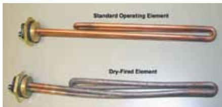
When an element is dry-fired, it loses its shape and becomes flexible to the touch as compared to a standard operational element that holds its firm shape. You can see the definite bend in the dry-fired element in the photo.
